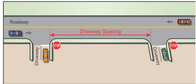
Access management can include increasing driveway spacing to reduce conflicts along the corridor. Source: FHWA.
