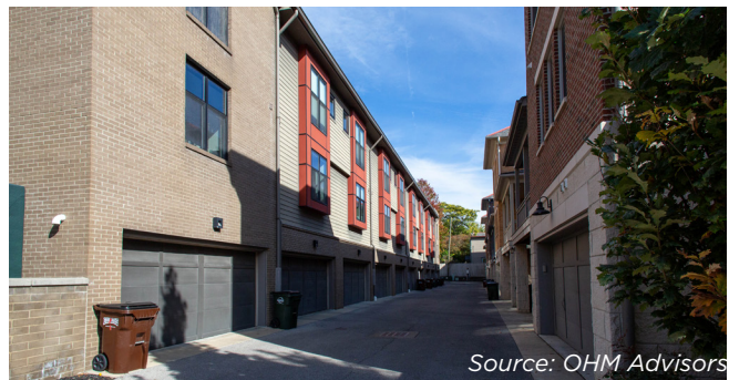
Source: OHM Advisors Townhomes can often "self-park" with tuck-under rear-load garage. On-street parking provides visitor spaces.
